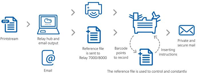
The reference file is used to control and constantly verify pages that are accurately folded and inserted.
